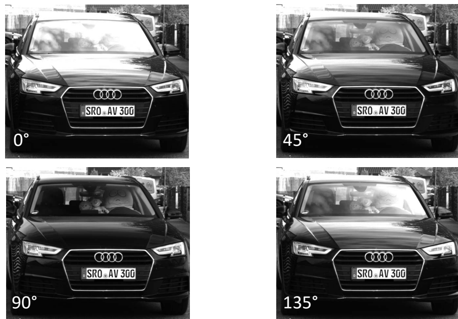
Figure 5: Polarization angle versus image brightness in sub-images
