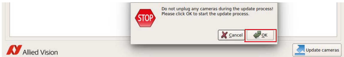
Figure 110: The command to update the firmware is confirmed
