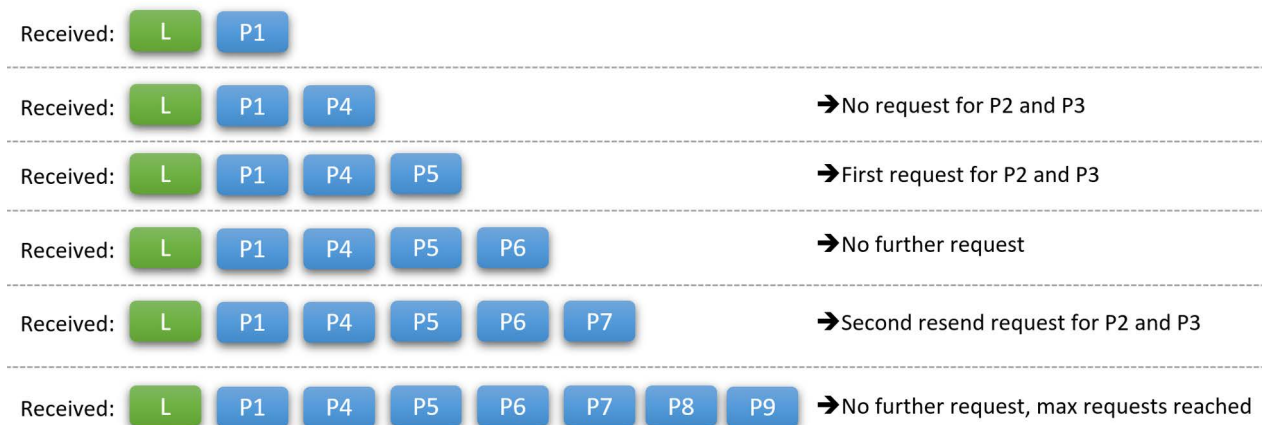
Figure 97: Controlling the resend of packets (example)
