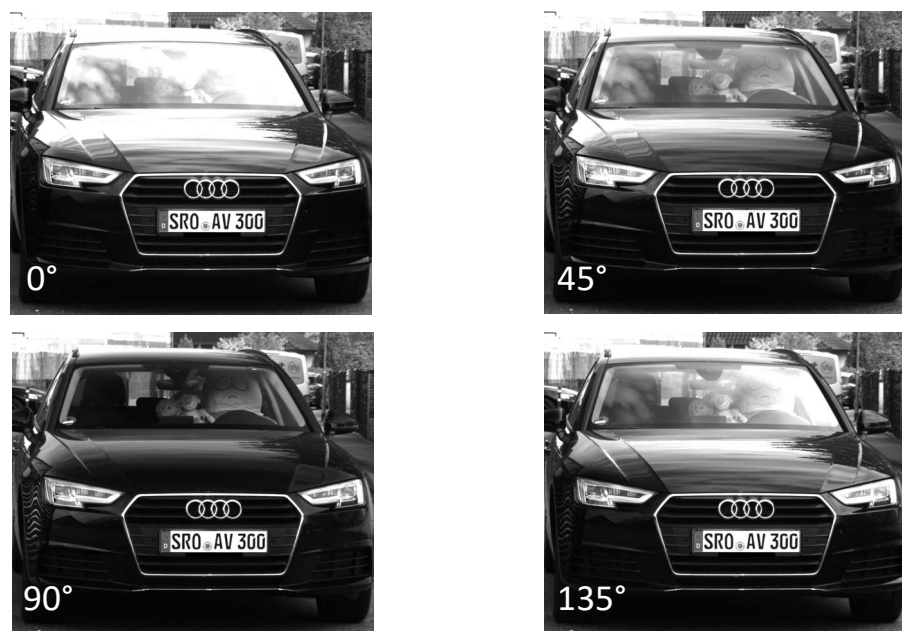
Figure 3: Polarization angle versus image brightness in sub-images
