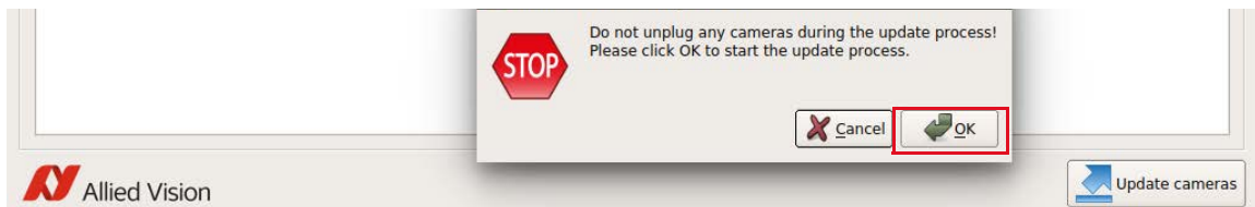
Figure 115: The command to update the firmware is confirmed
